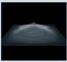
Anti-panic lighting: thanks to its square light distribution one luminaire is all it takes to illuminate spaces up to 130 m<sup>2</sup>.
