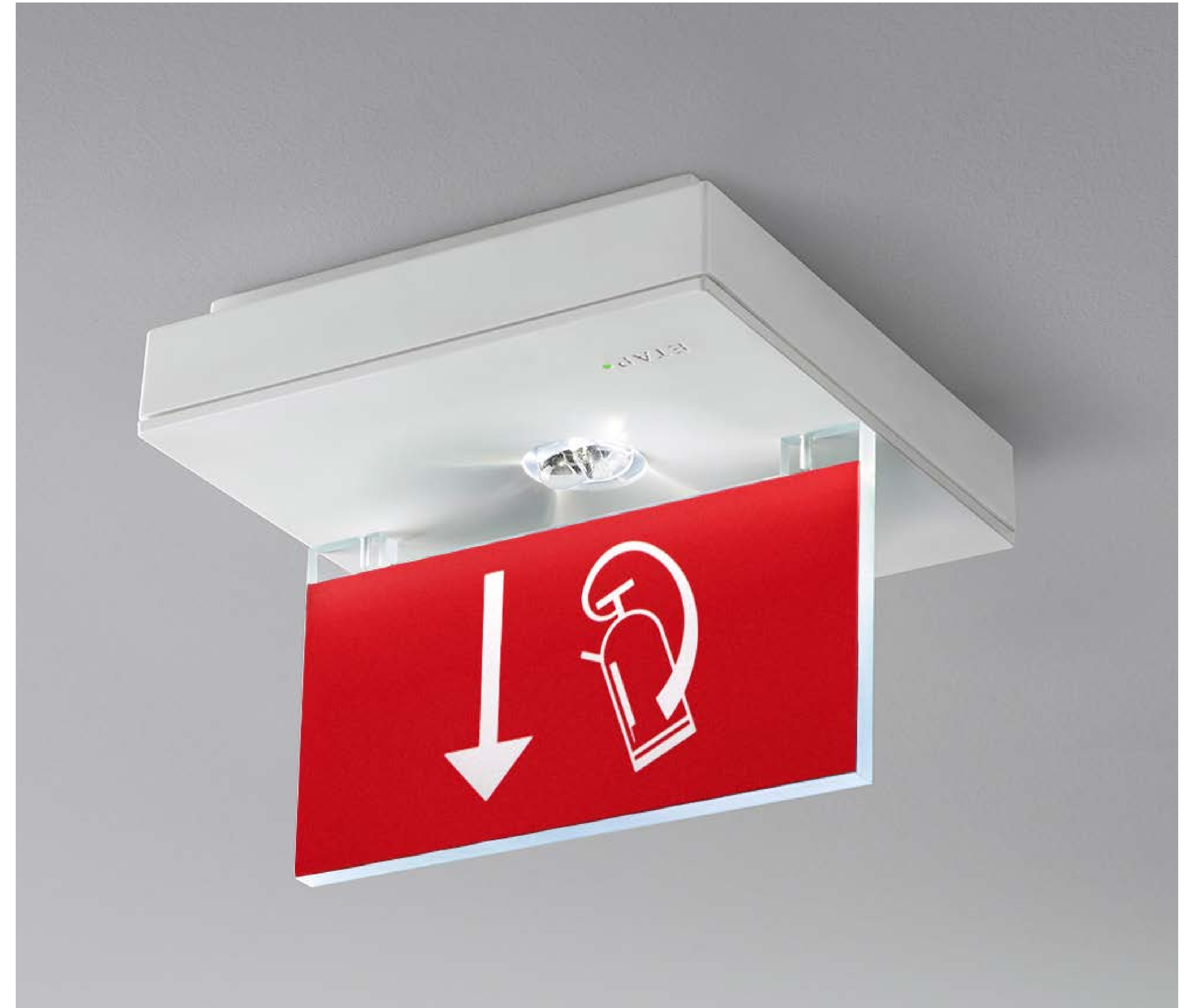
In the K1 with fire extinguisher signage, a special lens directs the light both into the pictogram and towards the wall/fire extinguisher.
